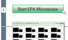
The EUROPattern Microscope automatically records the fluorescence images of all slides successively, without any further input from the laboratory staff. The fluorescence images can be viewed at once and verified directly at the monitor while the microscope continues with the image recording.
